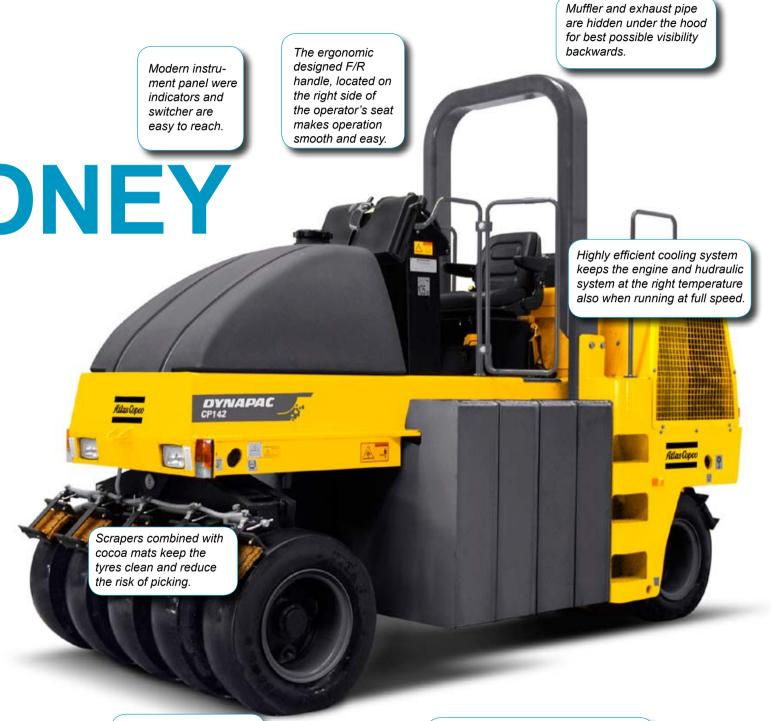
Unique modular ballast system gives direct visual control of the wheel loads.
