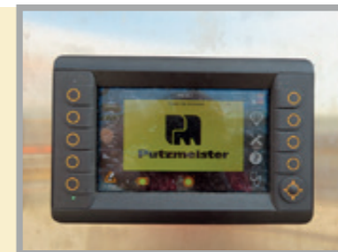
Highly intuitive control software via a multilingual colour display. Allows adjustment of additive dosage, indicates the concrete flow rate and troubleshoots errors
