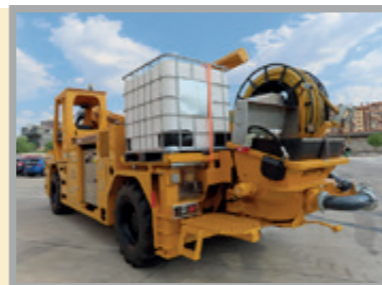
Putzmeister large diameter and long-stroke concrete pump that minimises pulsations and extends the useful life of wear parts
