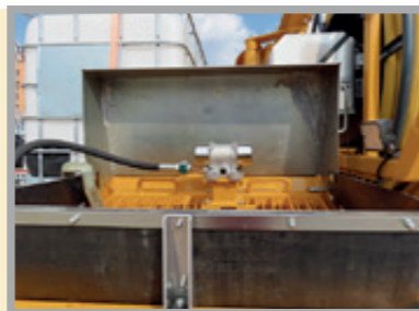
Hopper with agitator, electric vibrator and RFID security system on the grille. Pumping of steel or polymer fibres. Easy and safety to open for maintenance and cleaning.
