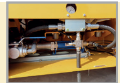
Screw additive pump with flowmeter to ensure a high-quality finish
