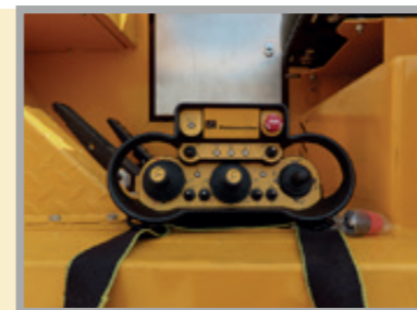
Dual radio and cable remote control for easy and precise management of arm movements
