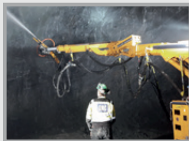
Optional Hydroscaling system for surface cleaning
