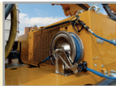
Built-in cleaning system with diesel and electric operation
