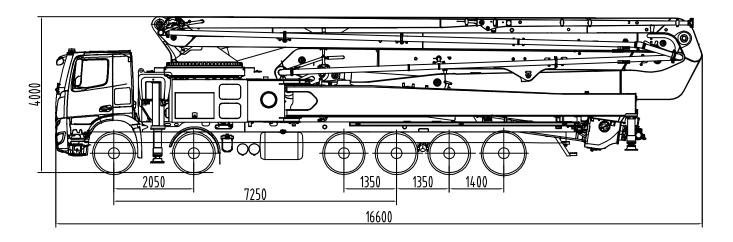
Note: Standard version. Dimensions and weights depend on truck, pump model and equipment. For illustration only.
